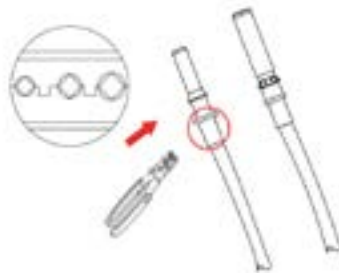
Crimp the contact pin to the wire
